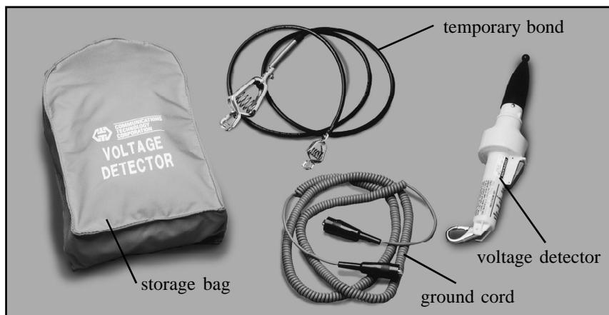
Figure 2: Voltage Detector and Accessories
